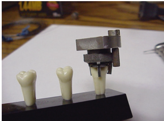
Fig. 8.6 Tooth clamping device and driving stage used to locate clamping device onto surface of the tooth
