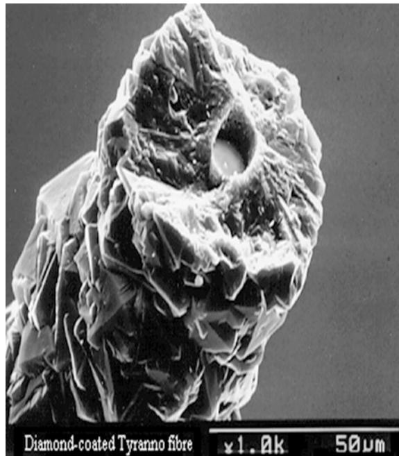
Fig. 5.2 Diamond coated Tyranno fibre (Ashfold et al. 1994; May et al. 1994, 1995; May 1995)
