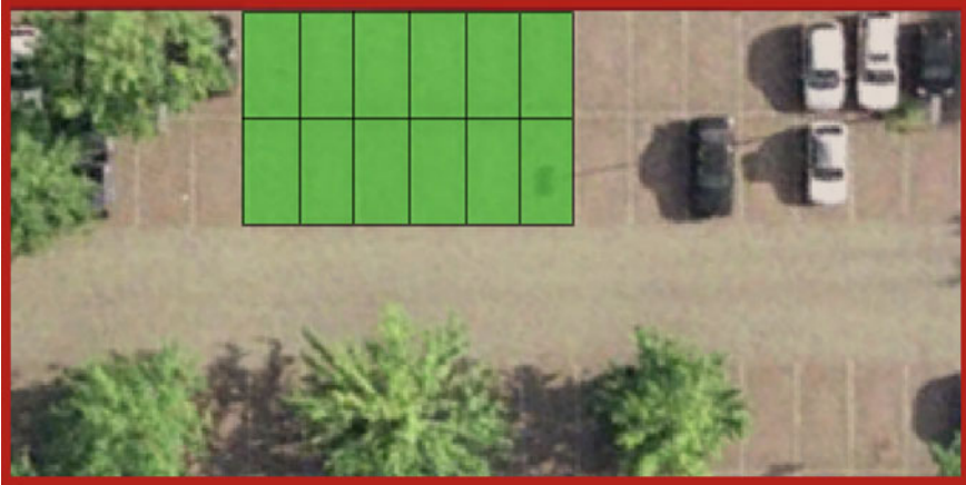
Fig. 3 The satellite image used to verify the mapped parking lots. Each of them is 5 \times 2.35 m
