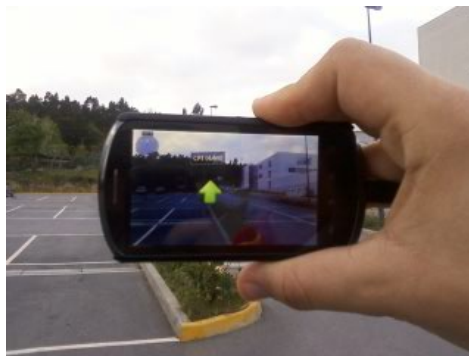
Fig. 3 Orientation system using augmented reality
