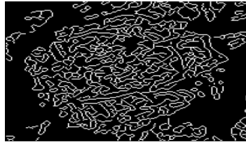
Fig. 8. Application of the CANNY detector on the ERS-1 image
