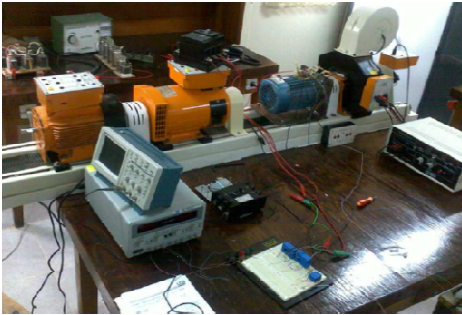
Fig. 5. The laboratory setup for induction motor stator faults experiments
