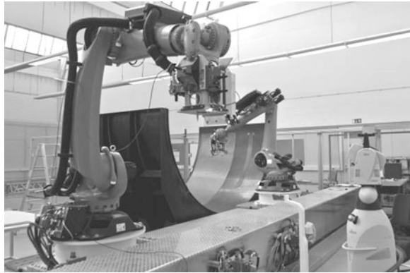
Fig. 8 External sensor guidance with laser tracker [5]
