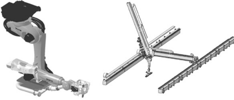
Fig. 3 Robot types in multifunctional cell (KUKA KR270 R2700, custom 6 DOF-Portal with KR240 arm)
