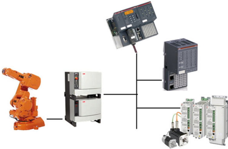
Fig. 7 The IRC5 robot controller with integrated AC500 PLC
