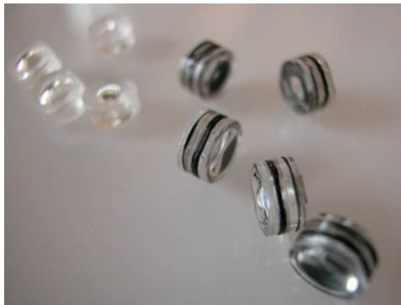
Fig. 3 Two types of cell phone lens assemblies. 4–6 parts are stacked on top of each other. Not all parts are transparent, diaphragms can be integrated as well
