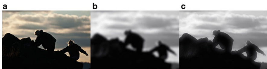
Fig. 2 High dynamic range compression and image enhancement using a single image under white light. (a) input image. (b) output of multi-scale retinex method. (c) output of our approach
