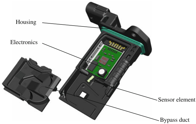
Fig. 1 Design of HFM8 air flow meter plug-in sensor
