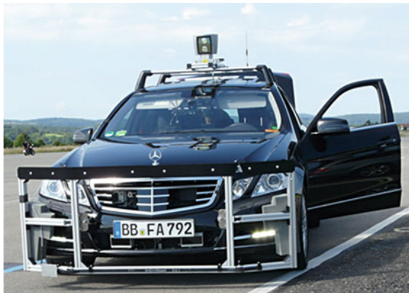
Fig. 1 A Mercedes E-Class is used as a demonstrator car. It is equipped with two laser scanners and a long- and mid-range radar. A Velodyne HDL-64E and a DGPS-module are used for evaluation only. A robust bumper is mounted for crash scenarios
