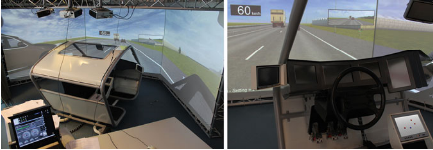
Fig. 1 Driving simulator used for the experiment. Photo on the right shows secondary task on the touch screen at the centre console
