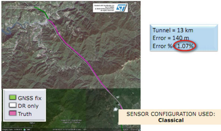
Fig. 13 Classical dead reckoning across a long tunnel, connecting the cities of Taipei and Yilan, Taiwan
