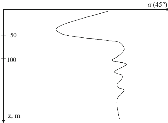
Fig. 28.36 Index of light dispersion (in arbitrary units) in a near-shore zone of the Bengal bay (adapted from MONIN (1978) [41]) © Nauka Publishing House, reproduced with permission
