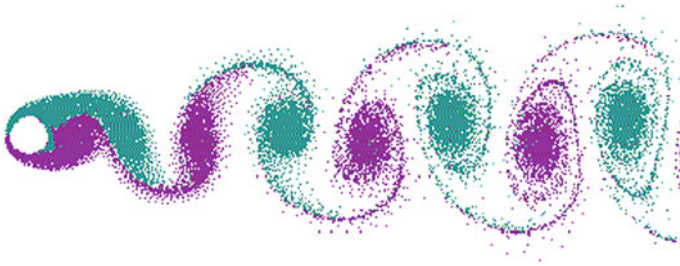
Fig. 28.9 VON KÁRMÁN vortex street behind a cylinder in uniform flow from the left ( http://www.icfd.co.jp/menu1/thermalconvection/therm.html )
