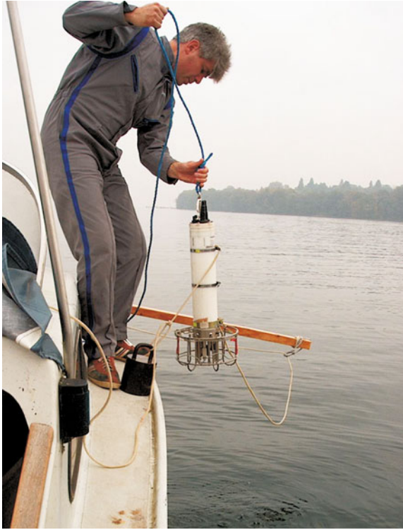
Fig. 28.22 Dr. Boris Chubarenko, making a vertical sounding in Lake Constance (2001) by CTD Idronaut Ocean Seven Model 316 of General Oceanics, Canada. The probe is equipped with the standard sensors to measure: pressure, temperature, conductivity, oxygen, pH, oxidation-reduction potential. Salinity is automatically calculated from conductivity, temperature and pressure values
