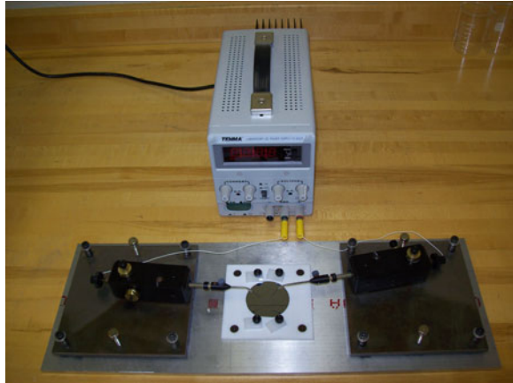
Fig. 3.31 Probe station setup for steady current exposure through Sn pattern
