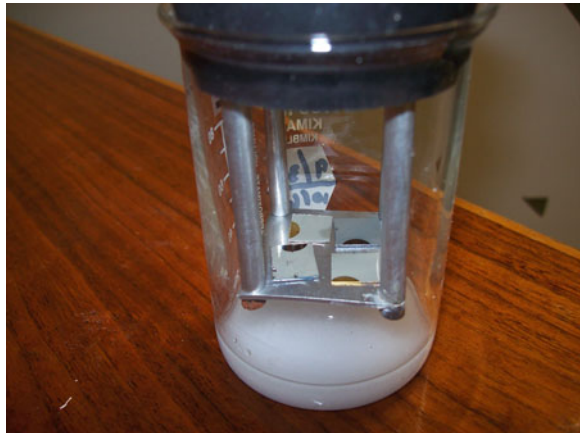
Fig. 3.7 Sputtered Sn film coupons exposed to saturated aqueous salt solution
