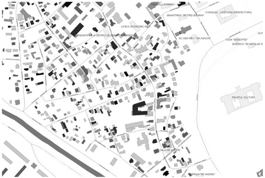
Fig. 5.7 The second scenario with a PGA value of 0.5g
