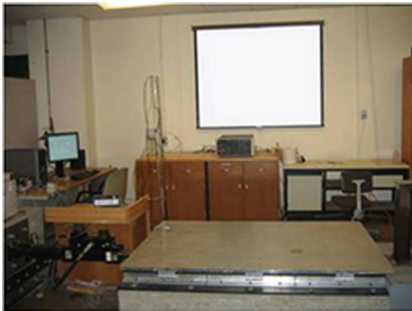
Fig. 21.2 1-D Shaking table used for research, education and outreach activities at Northeastern University
