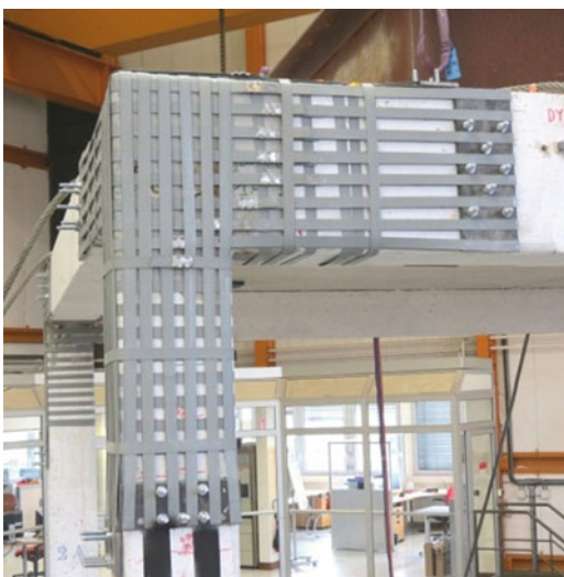
Fig. 11.6 PTMS strengthening at 2nd floor beam-column joints
