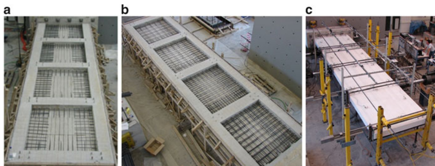
Fig. 16.2 Specimen no. 1: (a) frame with long starter bars and short dowels per option (a) along the top and one lateral side of each panel and the long dowels per option (b) along the other two; (b) two-way reinforcement placed in the new web; (c) specimen in testing position with actuators and sensors attached
