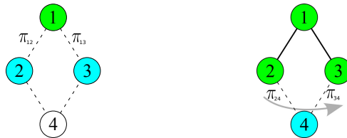
Fig. 5. A Cumulative Edges structure where (a) \Theta_{CE} = \{2; 3\} , \pi = \{\pi_2, \pi_3\} , \pi_2 = \pi_{12} , \pi_3 = \pi_{13} and (b) \Theta_{CE} = \{4\} , \pi = \{\pi_4\} , \pi_4 = E(\pi_{24}, \pi_{34})
