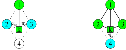
Fig. 8. A Naive Clustering structure where (a) \Theta_{\text{NC}} = \{2; 3\} , \pi = \{\pi_{(k,2)}; \pi_{(k,3)}\} and (b) \Theta_{\text{NC}} = \{4\} , \pi = \{\pi_{(k,4)}\}
