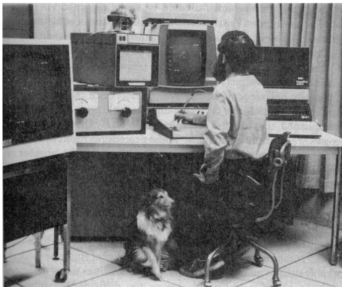
Fig. 1 The KINSYN III hardware. The human user was utilized as an integral part of the synthesis procedure. The user observed the current state of the design on the CRT screen and input directions for continuing the synthesis by way of a data tablet. As such, KINSYN may have constituted the first interactive computer aided engineering program. (Published by ASME, FIGURE 1 from [26], Journal of Engineering for Industry, Vol. 99 No. 2, by Rubel, A. J., and Kaufman, R. E., 1977.)
