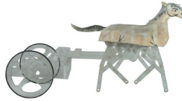
Fig. 8 NCKU's 8-bar-type horse carriage
