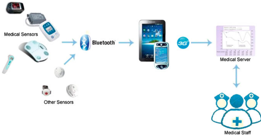
Fig. 1 Infrastructure for home telemonitoring systems
