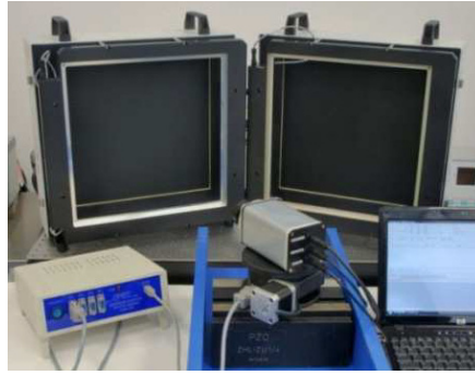
Fig. 19. Test stand for determining NUC correction coefficients and bad pixel identification in microbolometer focal plane array
