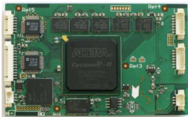
Fig. 7. Printed circuit board of FPGA-based digital image processing and control module
