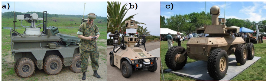
Fig. 10. Unmanned multi-purpose ground vehicles: a) Gladiator, b) MDARS, c) MULE (sources: Newton, 2011, Spawar Systems Center Pacific, Global Security)
