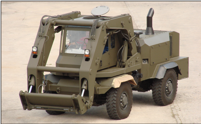
Fig. 1. WMI photography without front work tool, showing front working tool adapter (source: OBRUM)
