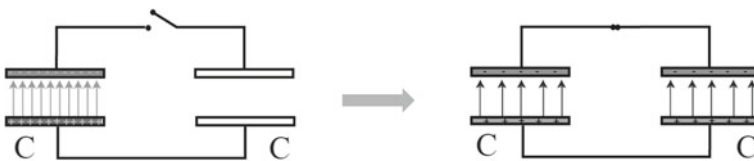
Fig. 56.1 The two capacitor problem. A capacitor is initially charged, the other uncharged ( left ). Then capacitors are connected so to share the electric charge ( right ). In this process half the electrostatic energy “disappears”
