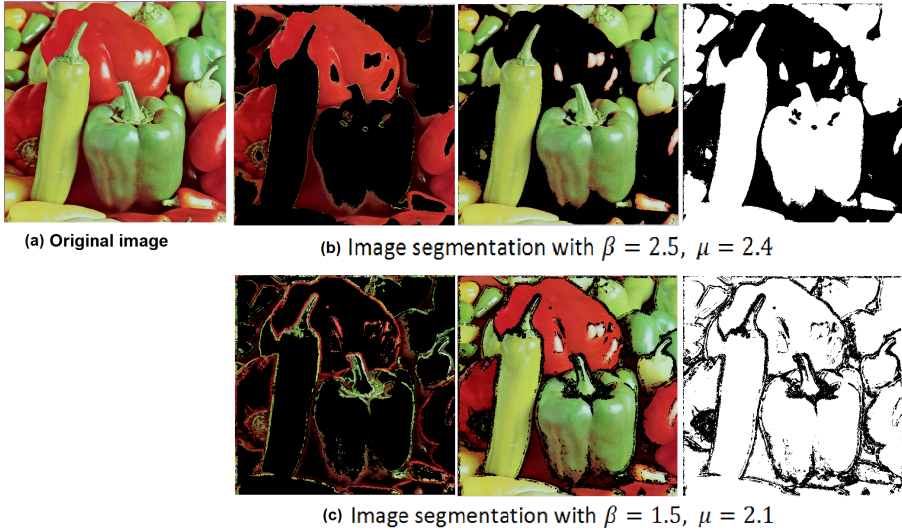
Fig. 3. Image segmentation by DCA-SI with different values of \mu and \beta
