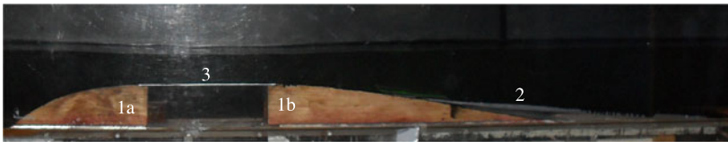
Fig. 8.4 Obstacle used for experiments: (1a) and (1b) curved parts motivated by airplane wing; (2) flat aluminum plate to further reduce flow separation; and (3) flat top aluminum plate to reduce wave tunneling effects
