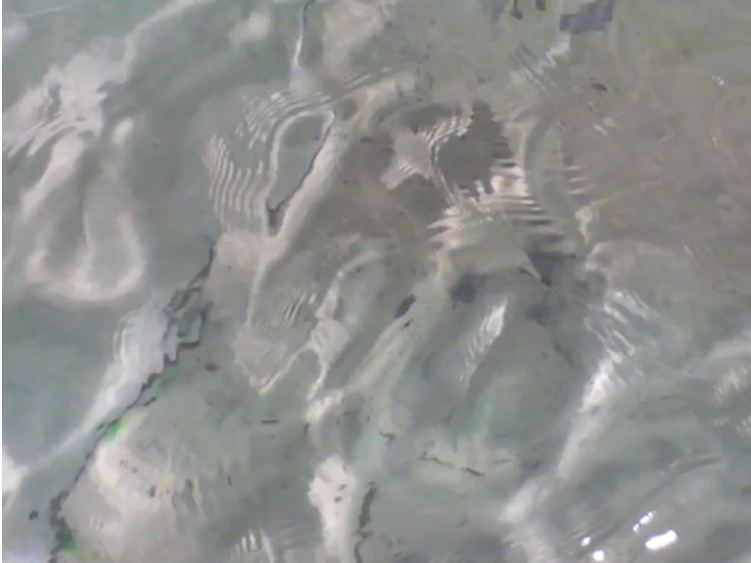
Fig. 7.5 Appearance of capillary waves for T = 0.4 s in the presence of a strong counter-current U
