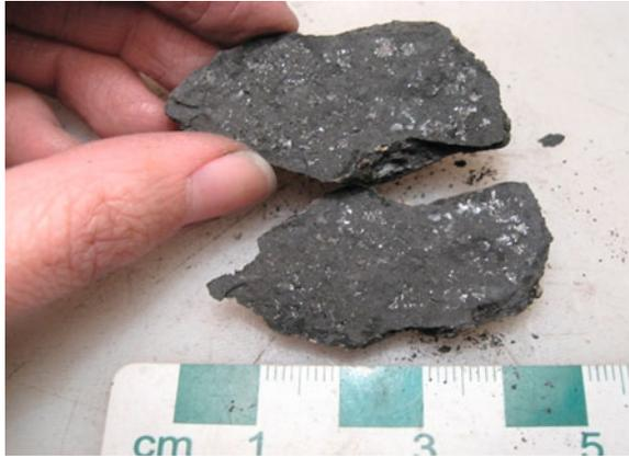
**Fig. 11** Aggregate particle from Quarry T with laminations propped open with gypsum
