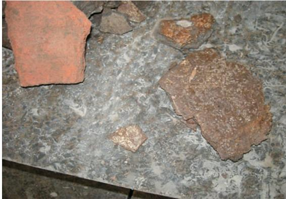
**Fig. 15** Chunks of shale bedrock extracted from beneath floor slab
