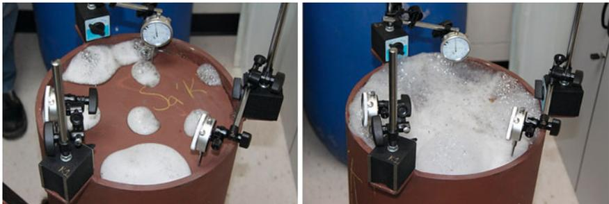
**Fig. 34** Foaming trial showing foam injected from the *bottom* of the sample escaping through and around the *top* plate
