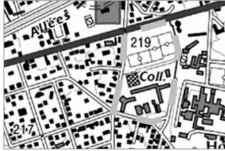
Fig. 3.5 The toponym, buildings, sports fields and footpaths are all functionally related to the complex object school (outlined with dashes )
