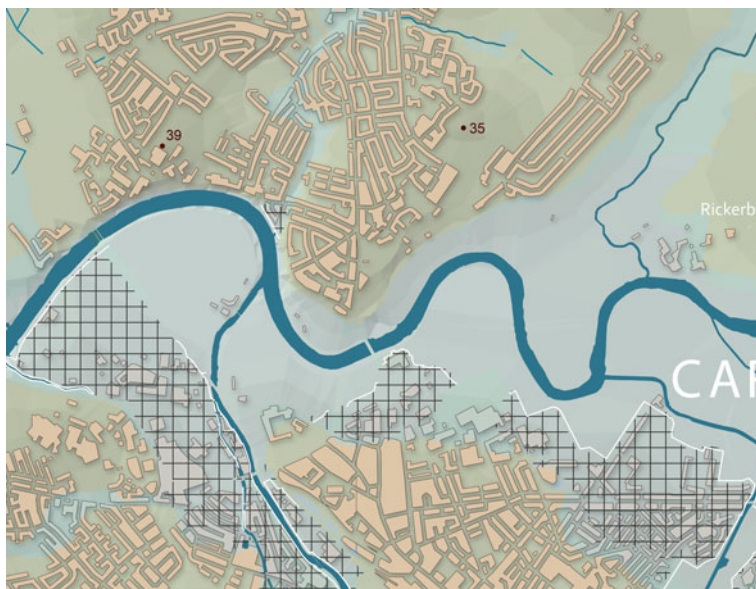
Fig. 11.13 OS VectorMap District combined with a height product to show flood risk in Carlisle. Ordnance Survey © Crown Copyright. All rights reserved
