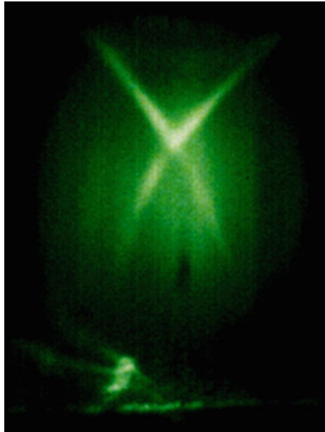
Fig. 6 The flow goes upward. The first shock composed of an expansion and a compression is observed
