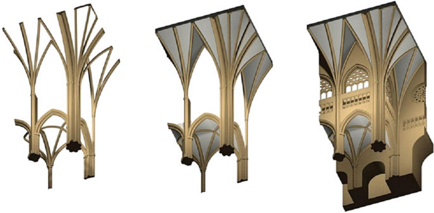
Fig. 22.3 Interior of the Bilbao Cathedral. The making of a computer model is similar to the physical creation of the cathedral. First, the columns and arches are constructed, followed by the vaults, piers and flying buttresses, and finally the walls, windows and ornaments. Rendering: authors
