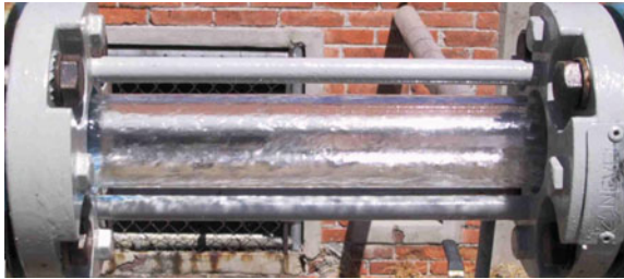
Fig. 2 Flow peephole photograph with annular two-phase flow
