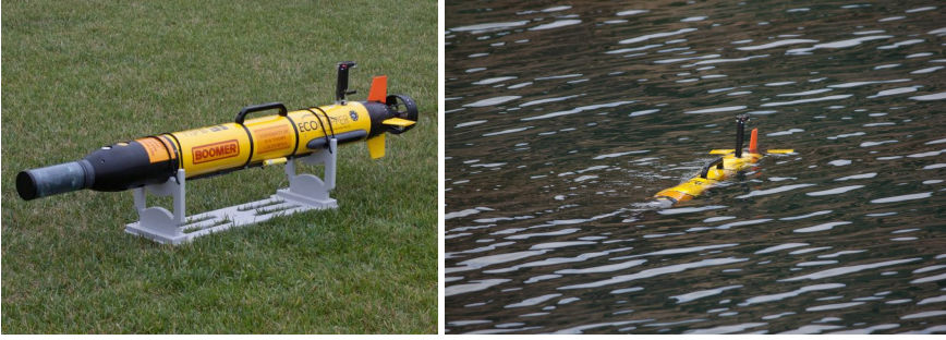
Fig. 1 YSI EcoMapper propeller-driven AUV used to perform bathymetric mapping experiments in Puddingstone Lake. The vehicle is equipped with an Imaginex Sportscan sidescan sonar for underwater imaging as well as a Doppler Velocity Log (DVL) for navigation.
