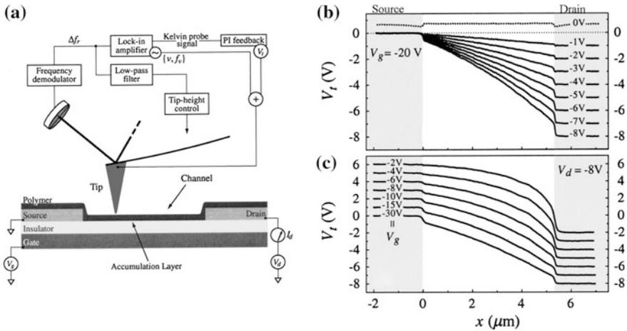
**Fig. 10.24** SKPM potentiometry measurements (a) measurement setup using an AFM probe head. Surface potential measurements on a P3HT TFT with Au contacts (b) in the linear regime with different drain biases, at a fixed gate bias, and (c) different gate biases at a fixed drain bias. (Reprinted with permission from [119]. Copyright (2002) American Institute of Physics)
