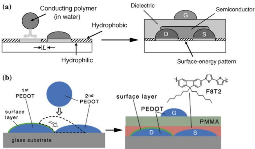
**Fig. 10.22** **a** TG/BC TFT printing, using substrate surface patterning to confine the water-based droplets of PEDOT-PSS forming the source and drain regions (Reprinted from [90]. Copyright © Materials Research Society 2003), and **b** sub-100 nm channel length TFTs using self-separating source/drain regions, formed by surface modification of the first droplet. (Reproduced from [66] with permission of John Wiley & Sons, Inc)
