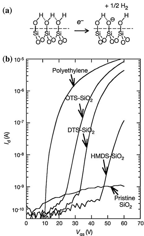
quenched by strong air-instability effects [36]. It was also noted that the sensitivity to silanol trapping reduced with increasing depth of the LUMO level.
