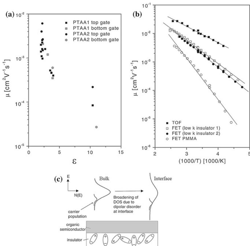
**Fig. 10.18** **a** Carrier mobility measured in PTAA TFTs as a function of the dielectric constant of the gate dielectric. **b** Temperature dependence of the mobility for different gate dielectrics, and **c** schematic illustration of the effects of disorder induced in the DOS at the semiconductor surface by a polar dielectric. (Reproduced from [105] with permission of John Wiley & Sons, Inc)
