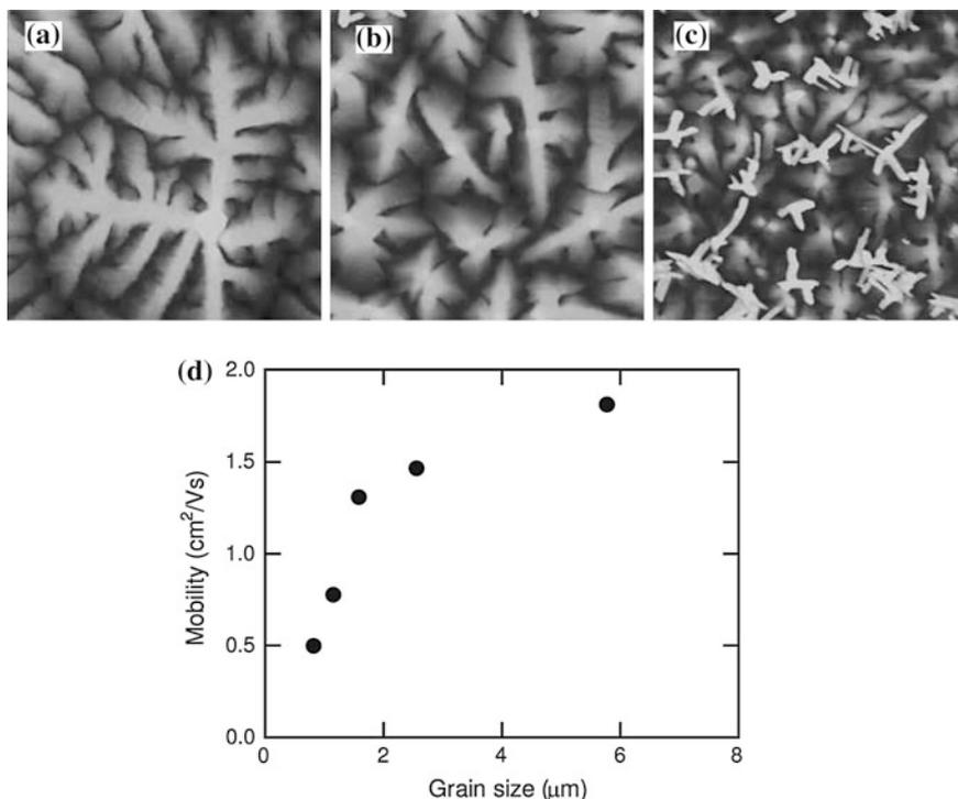
**Fig. 10.11** AFM images of pentacene grains grown at deposition rates of **a** 0.12 nm/min, **b** 1.2 nm/min, and **c** 12 nm/min. The AFM image size is  $5\ \mu\text{m} \times 5\ \mu\text{m}$ . **d** variation of mobility with pentacene grain size (Reprinted from [75], with permission from IOP Publishing Ltd)
