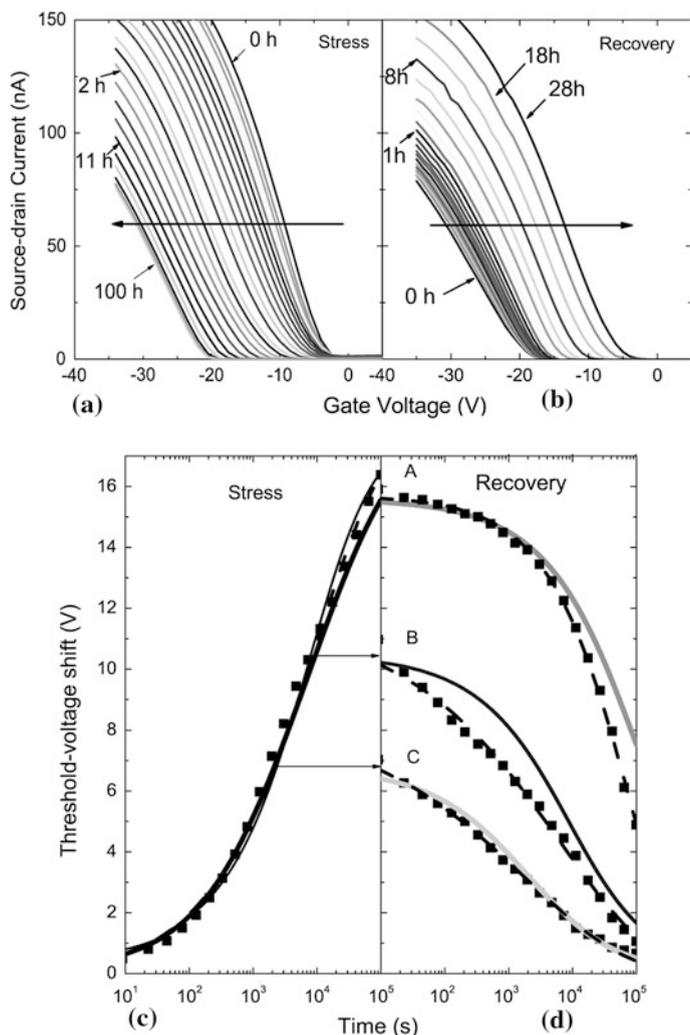
**Fig. 10.29** Transfer curves measured on a PTAA TFT as a function of time in air **a** with  $-20$  V gate bias stress, **b** recovery after removal of gate bias, **c** gate bias stress data (symbols), and fitted stretched exponential (dashed line), and **d** recovery data (symbols), and fitted stretched exponential (dashed line) (Reprinted with permission from [140]. Copyright (2010) by the American Physical Society)
