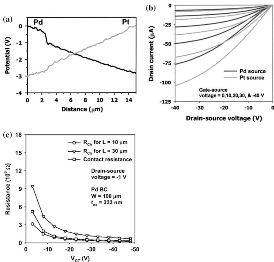
**Fig. 10.26** Measurements of pentacene TFTs with reversible Pt and Pd dual-metal source/drain contacts. **a** SKPM measurements. **b** output characteristics (Reprinted with permission from [123]. Copyright (2003) American Institute of Physics). **c** Channel and series resistance values as function of  $V_G$  on Pd-contacted BG/BC pentacene TFTs. (Reprinted with permission from [121]. Copyright (2006) American Institute of Physics)
