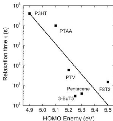
similar dependence of relaxation time on the HOMO level was also seen with the single crystal samples of rubrene, TIPS-pentacene and tetracene, albeit with a smaller slope than the data in Fig. 10.30 [142], indicating that these broad trends are quite common.
