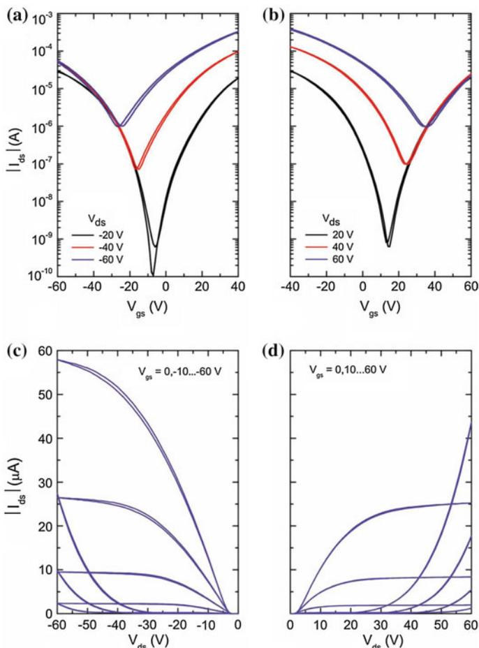
**Fig. 10.15** Transfer and output characteristics obtained from a PSeDPPBT ambipolar device. **a** and **c** p-channel, and **b** and **d** n-channel behaviour at negative and positive gate and drain biases, respectively. (Reproduced from [97] with permission of John Wiley & Sons, Inc)
