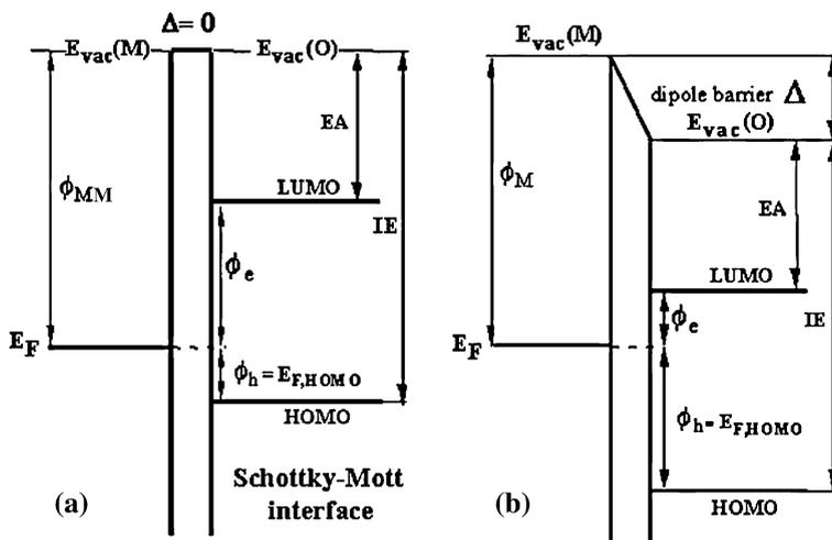
**Fig. 10.7** HOMO and LUMO band diagram of an organic semiconductor showing the band offset with respect to a metal contact **a** in the Schottky–Mott limit, and **b** with the formation of a surface dipole layer. (Reproduced from [39] with permission of John Wiley & Sons, Inc)
