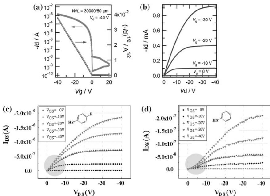
**Fig. 10.23** **a** Transfer characteristics, and **b** output characteristics of a Ph-PXX TFT (Reprinted with permission from [79]. Copyright (2009) American Chemical Society). Output characteristics of TIPS-pentacene TFTs, with Ag S/D contacts covered with different thiophenol-based SAMs, showing **c** good, and **d** poor injecting contacts. (Reprinted with permission from [114]. Copyright (2008) American Institute of Physics)
