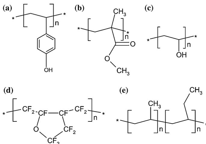
**Fig. 10.17** Chemical structures of common organic gate dielectrics **a** PVP, **b** PMMA, **c** PVA, **d** Cytop, and **e** PPCB. (Reprinted with permission from [101]. Copyright (2004) American Chemical Society)
