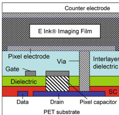
These TFTs had a mobility of  $0.01 \text{ cm}^2/\text{Vs}$ , an on:off ratio of  $10^4$ , and a threshold voltage of  $-5$  to  $-10 \text{ V}$ . The poor on:off ratio was attributed to the undefined channel layer, and, in later work, this ratio was improved to  $10^5$ – $10^6$  by patterning the semiconductor [57].
