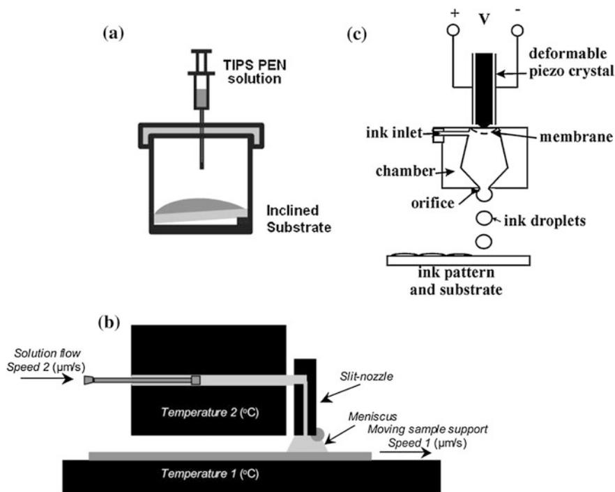
**Fig. 10.10** Semiconductor layer deposition by **a** drop-casting (Reprinted with permission from [63]. Copyright (2007) American Institute of Physics). **b** Zone-casting (Reprinted with permission from [65]. Copyright (2008) American Chemical Society), and **c** inkjet printing (Reprinted from [71] with permission of IEEE)
