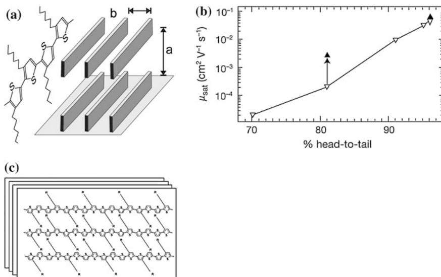
**Fig. 10.5** **a** Lamellar molecular ordering of regioregular P3HT (Reproduced from [28] with permission of John Wiley & Sons, Inc). **b** variation of hole mobility with fractional head–tail coupling in P3HT (Reprinted by permission from Macmillan Publishers Ltd: Nature [27], copyright (1999)), and **c** lamellar molecular ordering of PQT-12 (Reprinted with permission from [21]. Copyright (2004) American Chemical Society)
