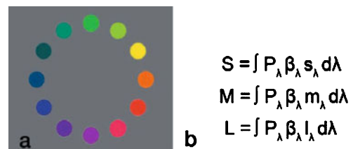
Fig. 6 a Color circle. b Calculation of absorption values S , M , L in the three kinds of rhodopsin of the cones with the absorption functions s_\lambda , m_\lambda , l_\lambda (Fig. 1b). The term P_\lambda \beta_\lambda stands for the stimulus (spectral power distribution of the radiation) emitted by the color papers of the color circle
