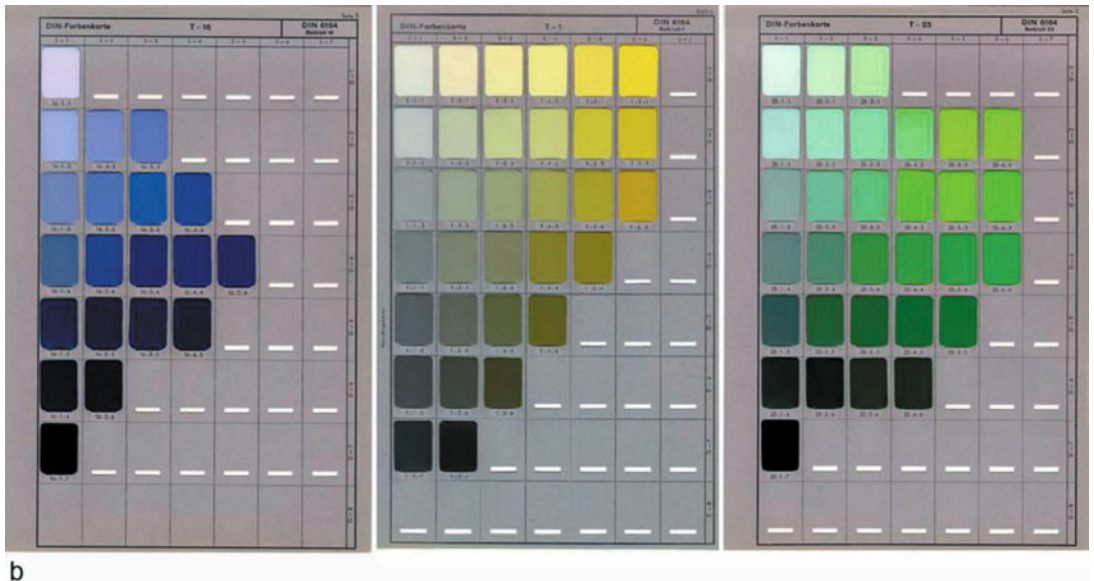
Fig. 3 Color charts taken a from the color atlas of Wilhelm Ostwald (Ostwald 1925) and b from the DIN-color atlas (DIN 1961)
