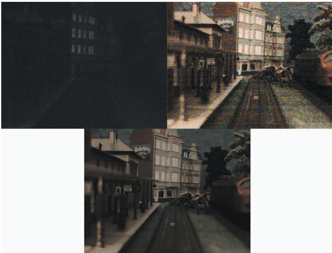
Fig. 2 Upper left: One frame from the original raw input data. Upper right: Contrast enhanced version with standard demosaicing. Lower panel: after noise reduction, including demosaicing and sharpening
