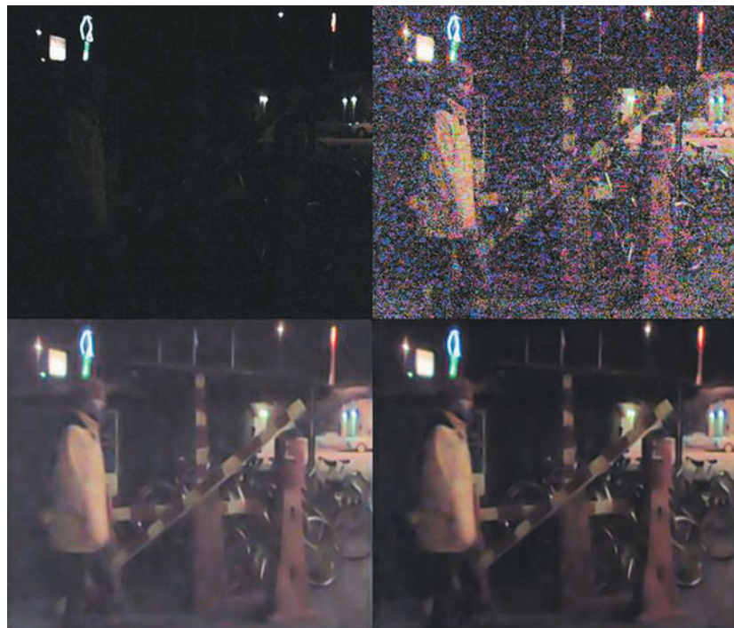
Fig. 1 Upper left: One frame of the original sequence. Upper right: Contrast enhanced version. Lower left: After noise reduction. Lower right: After intensity stretching
