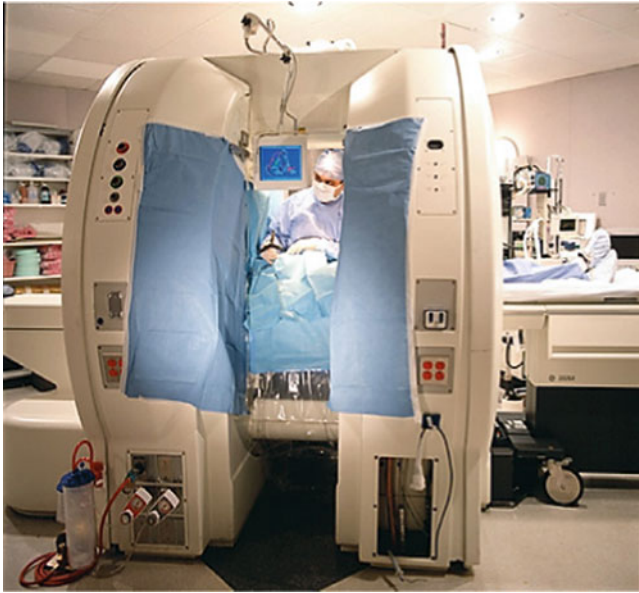
Fig. 1 General Electric Signa SP double coil 0.5 T magnetic resonance imaging scanner design that was installed at Brigham and Woman's Hospital in Boston in 1994. The surgeon is standing directly within the scanner and imaging updates can be obtained continuously during the procedure
