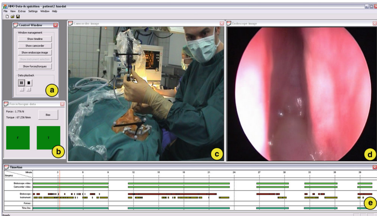
Fig. 1 Screenshot of the data acquire software during conventional endoscopic sinus surgery with explanatory notes: (a) control window, (b) force/torque data, (c) camcorder view, (d) endoscope image, (e) time line
