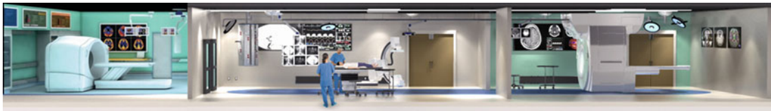
Fig. 1 Advanced Multimodality Image Guided OR (AMIGO). The middle room is an operating room with surgical microscope, angiography, ultrasound and optical imaging. The room on the left has a PETCT and on the right a 3T MRI which is ceiling mounted and can move into the operating room to image the patient on the operating room table (IMRIS, Winnipeg, Canada)
