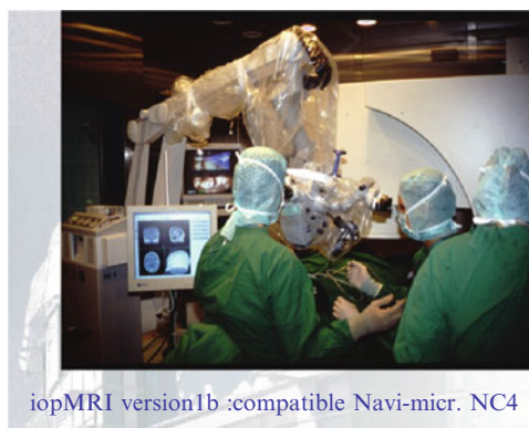
Fig. 3 ioMRI (version 1b) integration of the compatible navigation microscope Zeiss NC4 close to the modified diagnostic and therapeutic operation table
