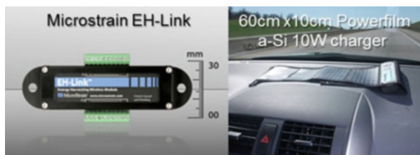
Fig. 13.13 Left , an energy harvesting-compatible, 8-strain gage wireless transmission node, and at right , a flexible, conformal 5 V output amorphous silicon photovoltaic system with sufficient power to power a single node from 40 min of sunlight per day
