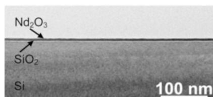
Fig. 5.21 Ultrathin neodymium oxide film on \text{SiO}_2/\text{Si} substrate deposited by an aqueous CSD process. Reprinted from [11] with permission from Cambridge University Press
