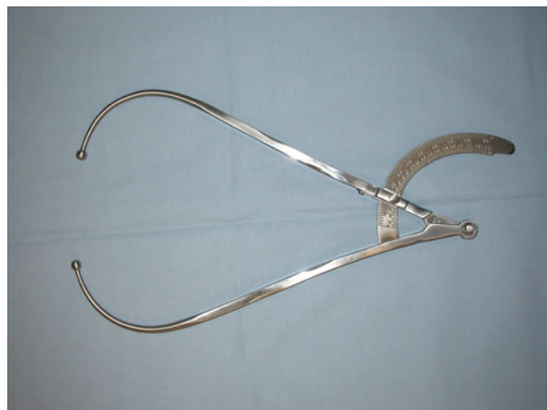
Fig. 1. Thorax-caliper made of steel, with a scale gauged in inches and centimeters. For validity of measurements the spheric ends of the branches must be moderately pressed against skeletal subcutaneous structures
