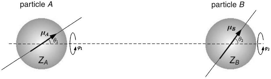
Fig. 2. Charge–dipole and dipole–dipole nanoparticle interactions. Interaction energy depends on the orientation of nanoparticle dipoles described by angles \theta_1 , \theta_2 , \varphi_1 and \varphi_2 in Eqs. (3) and (4)
