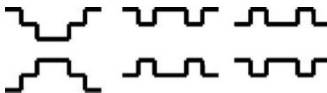
Fig. 1. Potential stepping in CSS nanocrystals (left), QDQW nanocrystals (middle) and “inverse” QDQW nanocrystals (right)
