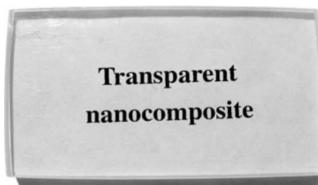
Fig. 9. Photograph of a bulk nanocomposite containing 20 wt% ME-capped ZnS (sample thickness: 4 mm). Reproduced with permission from [64], © 2006 Wiley–VCH
