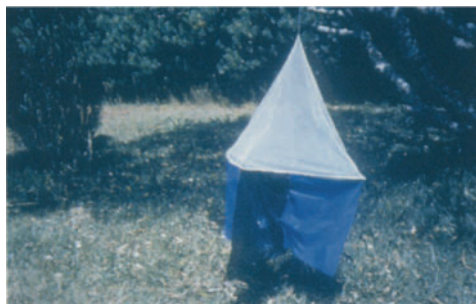
Fig. 267 Biconical tsetse trap [4]
