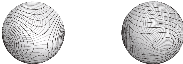
Figure 2.9: \mathcal{M} for the planar three-body problem is the shape sphere. The Newtonian potential determines a Morse function with five critical points, shown here for the case of equal masses (left) and masses 1, 2, and 10 (right).
