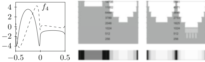
FIGURE 6.6. Real and imaginary part of f_4 and associated admissible meshes of Algorithm 3 (left m = 1 and right m = 3 )
