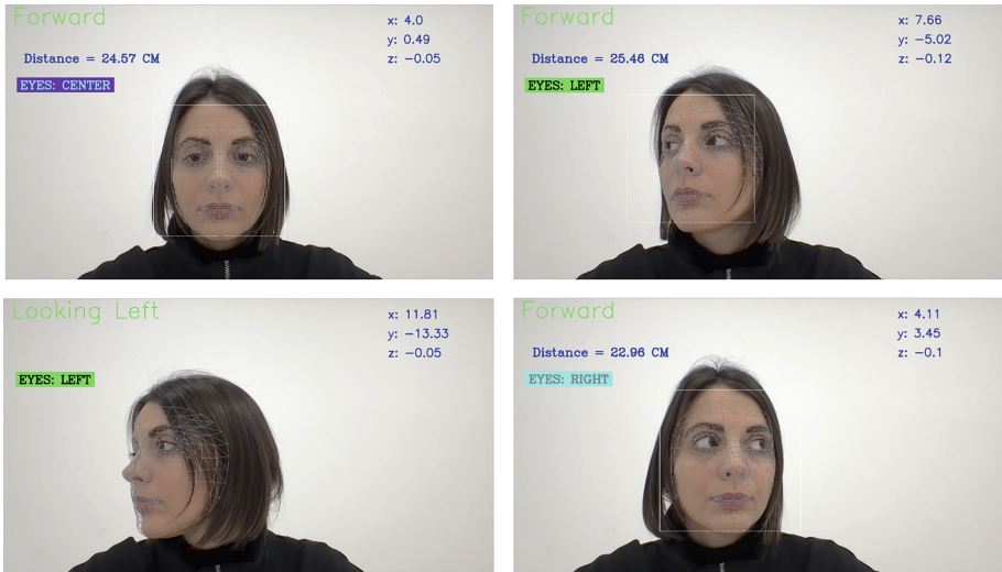
Fig. 3. Biometric-based measures to perform drowsiness detection, distance estimation, gaze position and head rotation.
