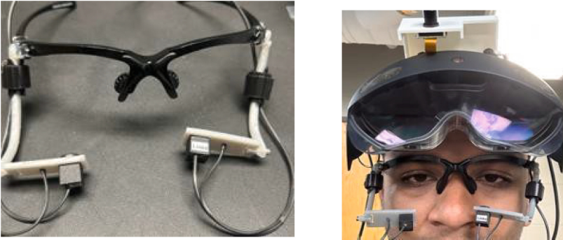
Fig. 2. Dikablis eye tracker & HoloLens and Eye tracker placement.
