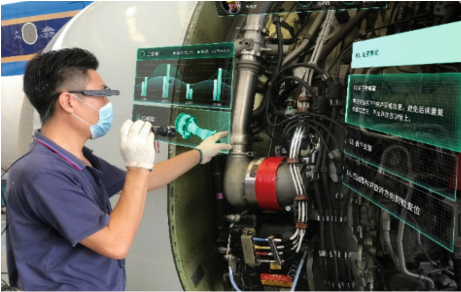
Fig. 3. Wearing AR glasses, the aircraft maintenance personnel can receive real-time guidance and diagnoses from experts (Source: Based on [32]).
