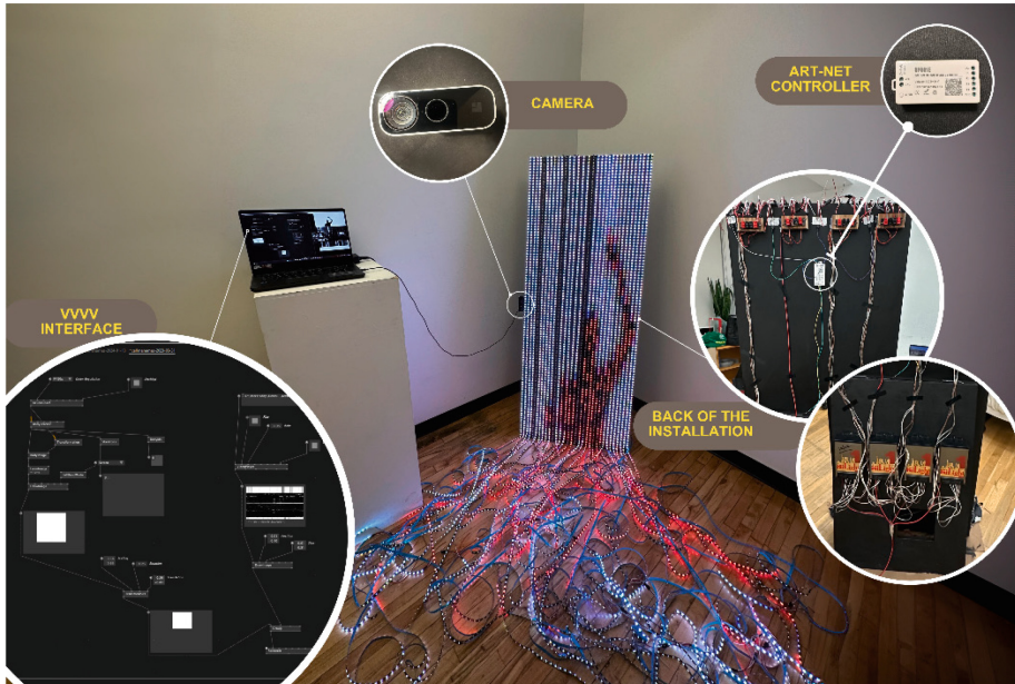
Fig. 6. Photo of the final “Data Shed” installation, including the labeled hardware and software; latent data is captured and presented within the piece dynamically.
