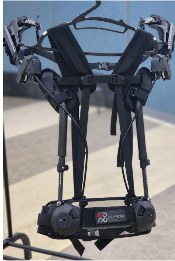
Fig. 1. CDYS shoulder exoskeleton (Crimson Dynamics Technology Co. Ltd., Dalian, China)
