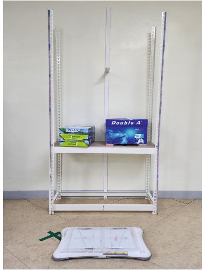
Fig. 3. Experiment setup to simulate the holding tasks in industry: Wii balance board placed in front of the custom-made storage shelf
