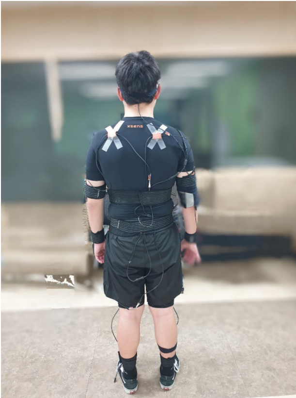
Fig.4. Wearable Xsens MVN system for measuring subject's shoulder ROMs
