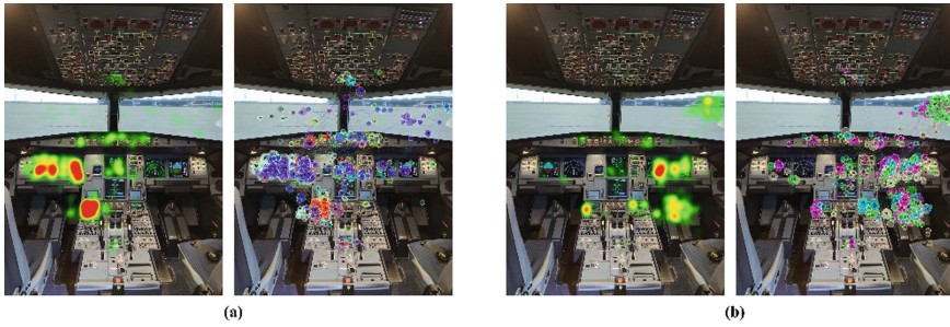
Fig. 11. Eye-tracking Visualization Results During Approaching Stage. (a) heatmap and gaze plot for PF. (b) heatmap and gaze plot for PM.
