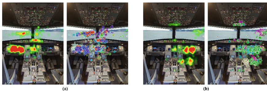
Fig. 13. Eye-tracking Visualization Results During Landing Stage. (a) heatmap and gaze plot for PF. (b) heatmap and gaze plot for PM.
