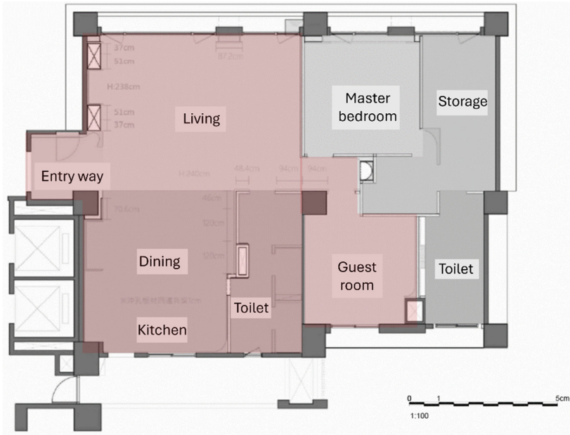
Fig. 2. Figure is the interior design diagram of the plan configuration. The sound field evaluation of the open plan includes the living room, dining room, kitchen and adjacent toilet and guest space. The indoor sound field evaluation is the area marked with red color blocks.
