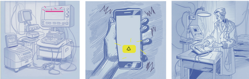
Fig. 8. Proposed innovation: the alarms and their log put on a separate portable screen (e.g., a mobile phone), which will always be at the doctor's office and signal him about critical situations with an audible alarm and an alarm screen. Design team Angelina Kablova, Anastasiia Mareva, Veronika Volkova.
