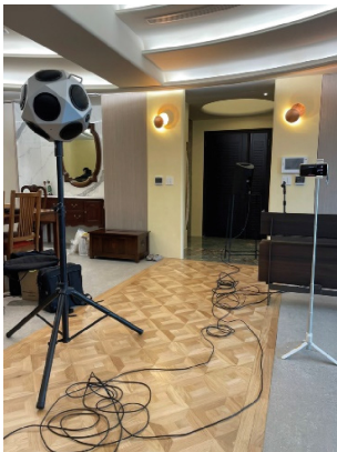
Fig. 7. The reverberation time T30 measuring system was collected by B&K 2755-A, 4292-L-001 and Type-4966 measurement instrument
