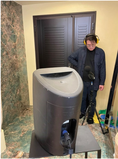
Fig. 10. Sound insulation performance of the door sound insulation parameter value ( D_{nT,w} \geq 35 dB) between the sound source side and the sound receiving side.
