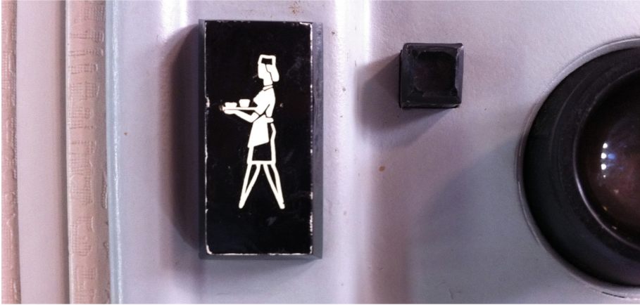
Fig. 4. Detailed icon of Passenger Call Button in a Soviet aircraft [36]
