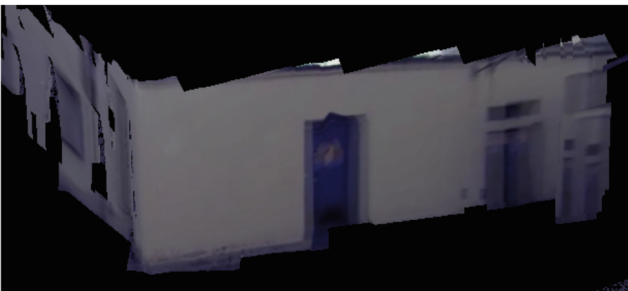
Fig. 7. Two images that overlap imprecisely create the illusion of fuzzy discontinuities, like at the frame of the blue doors in the image. (Color figure online)
