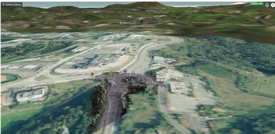
Fig. 5. Representation examples of 3D terrain elevation with orthophoto imagery [7] as base layer and LiDAR pointcloud from mobile mapping [1].
