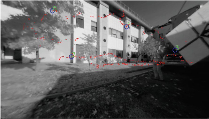
Fig. 6. All the correspondences found between the image and the 3D geometry as red dots. Selected correspondences are rendered with blue circles. The greyscale version of the image is rendered in order to better highlight the correspondence points (from [9] (Color figure online)).
