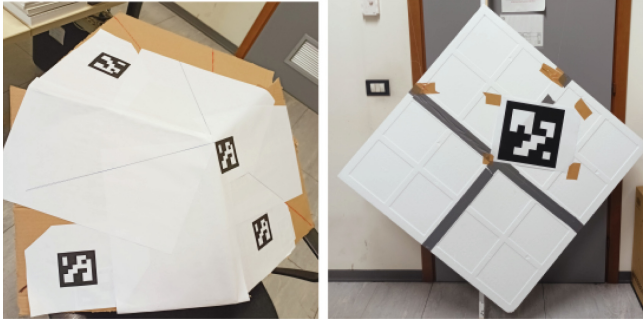
Fig. 2. Left: preliminary version of the target; Right: refined target used with our system (from [9]).
