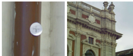
Fig. 3. Example of a retroreflective target (left) and natural point (right) [44].
