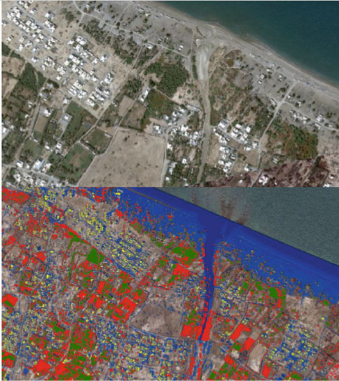
Fig. 4 Impact of the Shaheen cyclone on the Al-Batinah region. Top: before, bottom: after the cyclone. Red: farms degraded by cyclones. Blue: water inundation intensity
