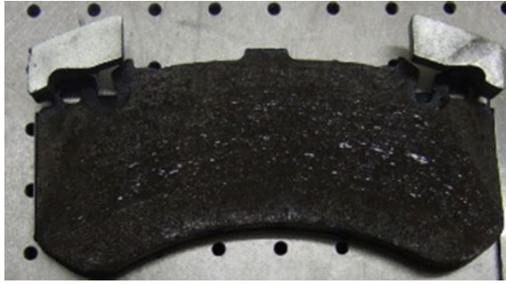
Fig. 6.38 Mass added to back-plate of pad shifts frequency and changes mode of vibration
