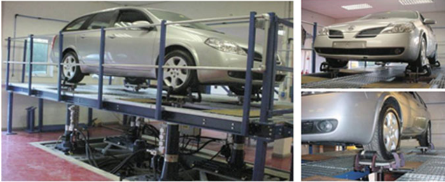
Fig. 5.26 Four poster dynamic test rig
