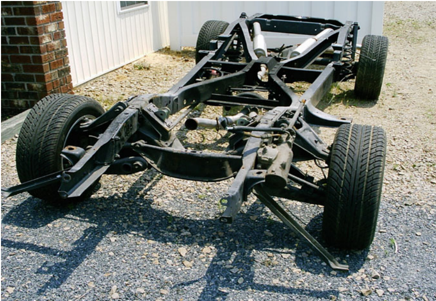
Fig. 5.1 Typical small truck chassis ( Source Christopher Ziemnowicz, licensed under [CC BY-SA 2.5], via Wikimedia Commons from Wikimedia Commons)
