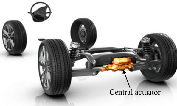
Fig. 4.60 The general assembly of a single (central) actuator (Source ZF Friedrichshafen AG)
