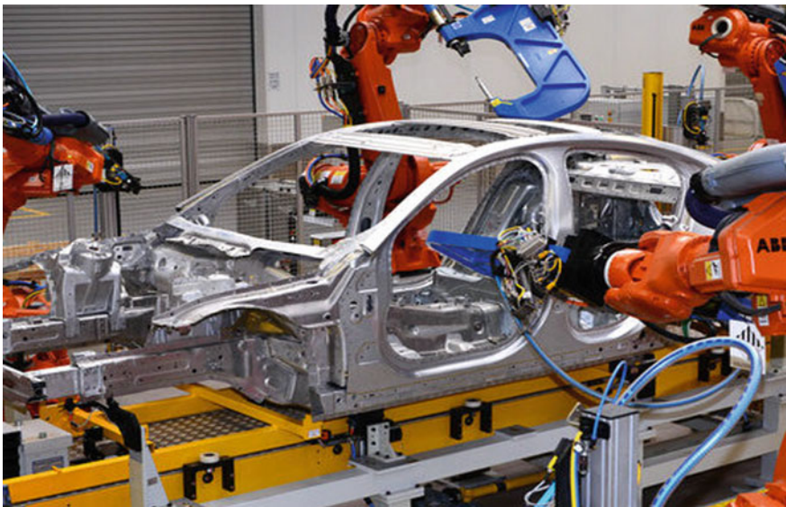
Fig. 5.2 Aluminium integral body shell during manufacture ( Source Jaguar Land Rover Ltd.)
