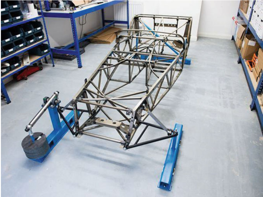
Fig. 5.7 Torsional test of space-frame chassis ( Source Simpac Engineering Ltd.)
