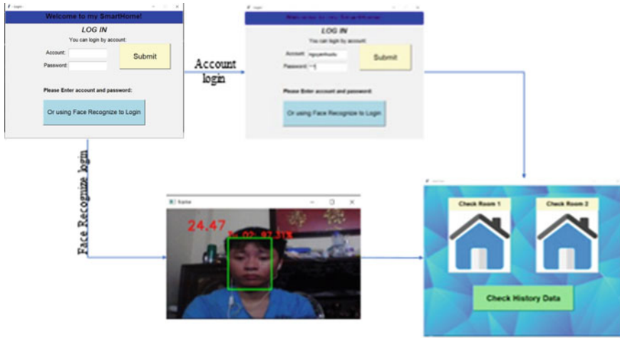
Fig. 5 The control interface of IoT system
